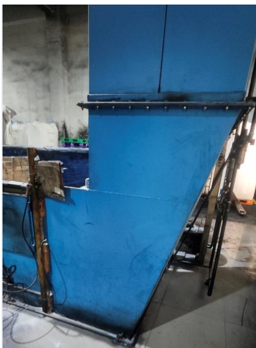
2#炭黑解包设备及废气收集罩
